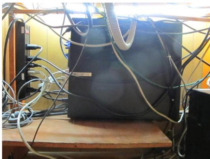
industrial computer with a solid-state drive. (Work still continues on making the remote station available to any Skyview member that wants to use it. I'm not happy with its current configuration. Stay tuned) To the left is an AC power strip that's connected to UPS power. Along the top of the picture is the copper pipe that is used as the station ground bus. All major equipment is tied to this pipe.
