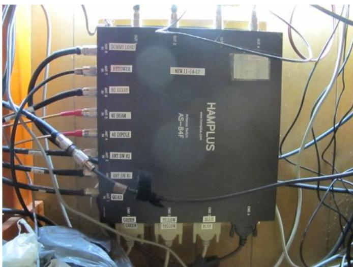
the left. Cabling from the four selector units connect on the bottom. The plastic bags you see on the bottom left hold oil filled dummy loads. I connect these up to antenna ports on the switch if one or two antennas are out of service. This way, if someone tries using an antenna that's not there, no damage is done.
